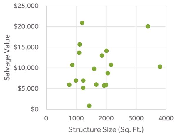
Figure 6: Relationship between Structure Square Footage and Value of Materials Salvaged from Deconstruction Project Data Set
